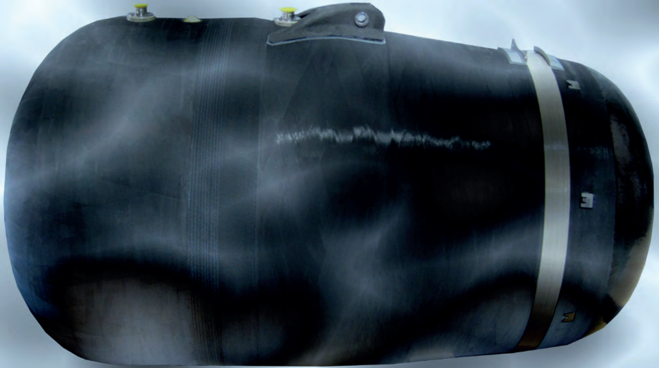
1 | A350XWB Potable Water Tank ©Matthias Gondeck
